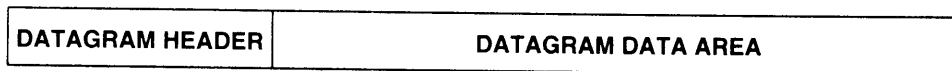
Figure 7.2 General form of an IP datagram, the TCP/IP analogy to a network frame. IP specifies the header format including the source and destination IP addresses. IP does not specify the format of the data area; it can be used to transport arbitrary data.
